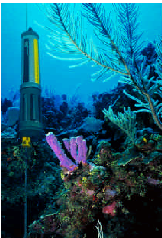
Figure 1. YSI 6600 sonde deployed in a coral reef for long-term data collection.
