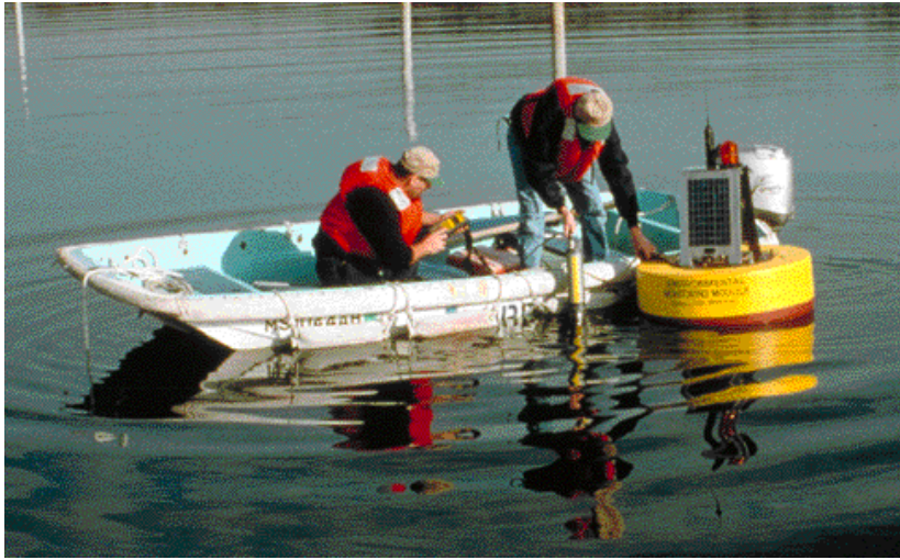
Buoy-Based Real-Time Data Acquisition of Coastal Water Quality
