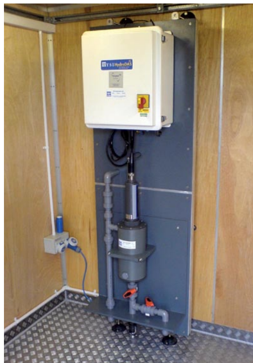
The compact HydroSAM provides long-term water quality monitoring for intake protection with less maintenance than larger systems. Shown here inside a protective shelter upstream of the water intake.
