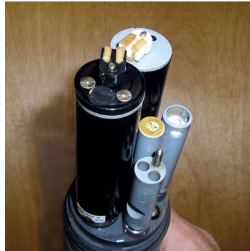
Close-up of sensors. The two larger optical sensors have integrated wipers to keep them free of fouling from organic compounds.
